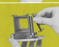
Insert the empty spool on the right side by pushing it up against the forked spring as shown. Slip the opposite end in place.
