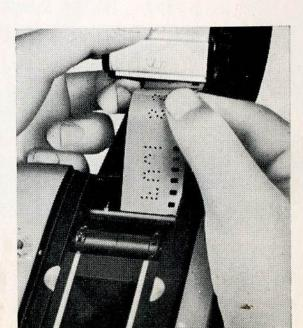
b) Be sure to have the sprocket gear (28) engaged into perforation of film. By turning the spool with finger, wind the film one complete turn on the spool.
