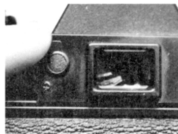
Built-in shutter blind to prevent extraneous light from entering finder is useful; it's controlled by lever at back.
