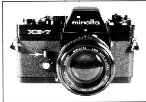
With its fixed pentaprism and compact "vertical" shutter, the XE-7 is low-profiled. Self-timer (arrow) shields its own release.
