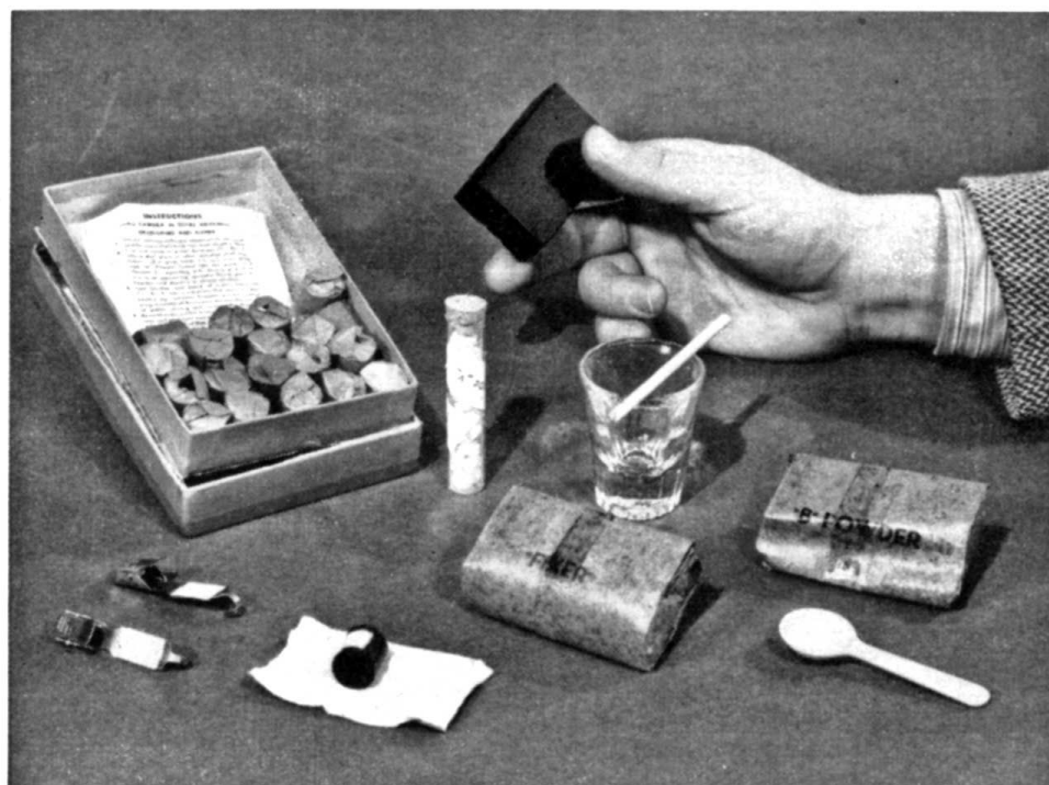
Complete photographic kit developed for use by the O.S.S. during World War II consisted of matchbox camera (in hand), film, processing equipment, chemicals.
