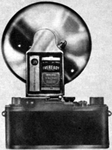
B-C flash circuit using miniature "B" battery and electrolytic capacitor was first used in Jen-Flash II in 1949.
