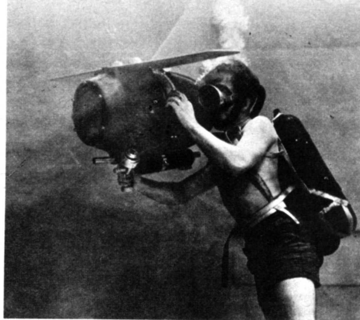
Diver-photographer adjusts focus and lens diaphragm of Aquaflex 35-mm underwater motion picture camera, of French manufacture.
