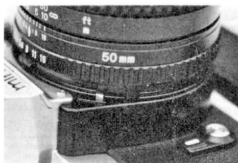
The small silver pin actuates the meter display when in shutter-priority mode.
