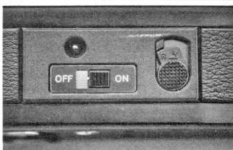
Auto Winder D controls; LED cycling lamp remains on at end of film.
