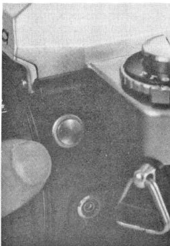
Items on side of lens mount, top to bottom, are: lens release button, sync terminal, depth-of-field preview button.
