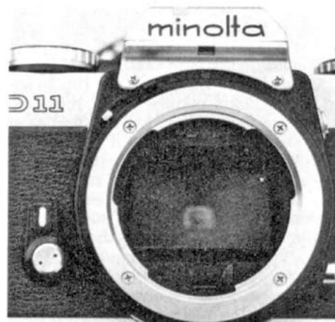
The reflex mirror of the Minolta XD-11 is oversized, preventing image cutoff.
