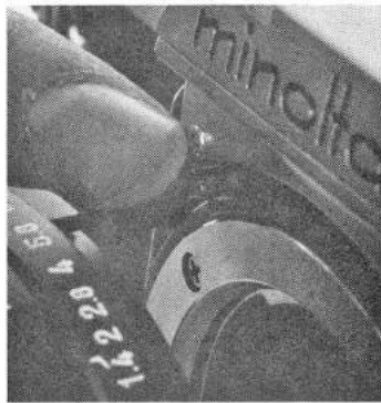
Spring-loaded rim-driven lug keys lens aperture to camera—same system used on all Minoltas SLRs since SRT-101.
