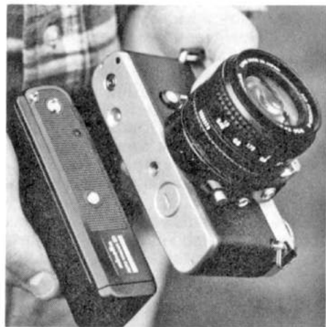
The drive is self-aligning when the locating pin is engaged in the hole in the baseplate.
