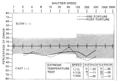
Suggested USA (formerly ASA) shutter accuracy standards are shown by shaded area. Higher speeds have more tolerance.
