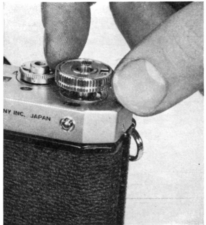
Close-up of manual film wind knob shows it in elevated position. This is for auxiliary use only; ordinarily film is advanced, shutter cocked by means of rapid wind lever on camera's baseplate. Knob is easy to operate.
